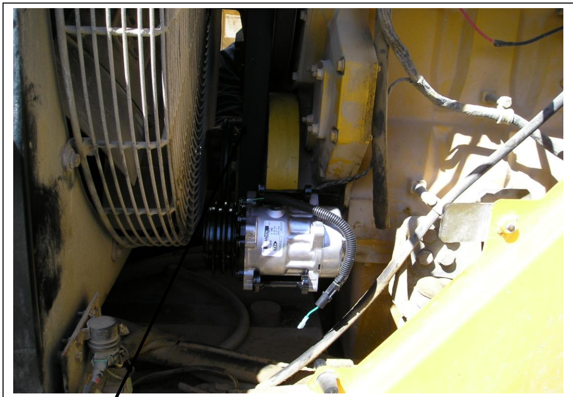
Pulley bolts onto the crank using longer M12 bolts in place of the original bolts.
