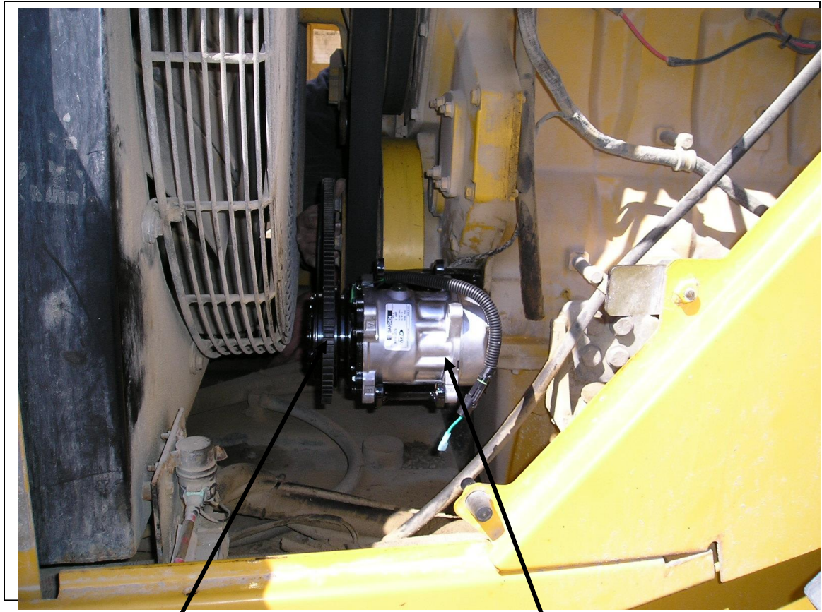
Belt on compressor and on crank pulley.
